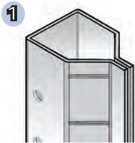
6-Bend Structural roll-formed vertical framing member
